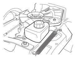
**Rider 15T** Fill if necessary with engine oil SAE 10W/40 (class SF–CC).
